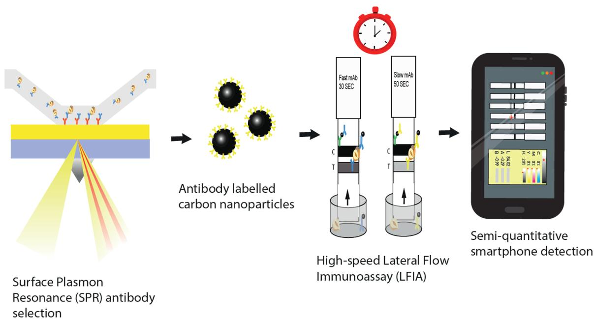
**Figure 1:** Graphical illustration of an SPR high-speed lateral flow immunoassay method incorporating smartphone detection.
